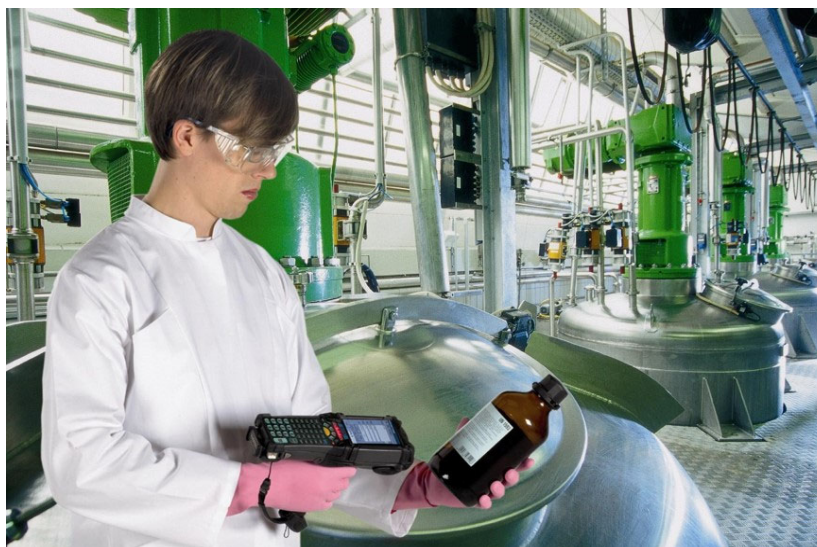
↑ An Ex certified mobile computer – but always remember: is this device suitable for the relevant zone?
