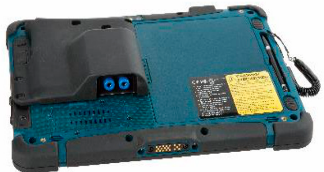
BARTEC Agile X (Zone 2) with mounted HART add-on module
